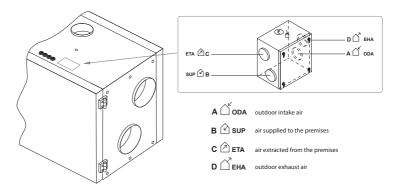
Fig. 8. Air duct marking
