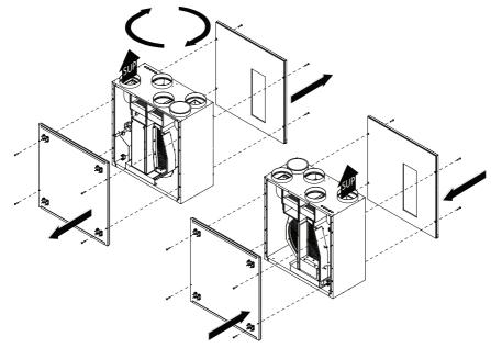
SUP – Supply air duct connection.
