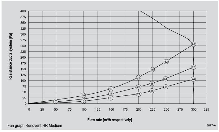
Note: The value stated in the circle is the capacity per fan (in Watt)
