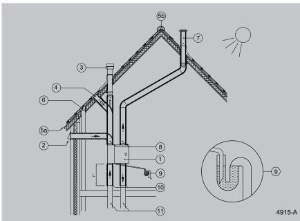
Arrange the exterior air supply from the shadowed side of the dwelling, for instance from the wall or overhang. If the outdoor air is sucked in from under the tiles, it must be ensured that no condensation develops in the roof boarding and no water can run in. Ventilation air can be sucked in from under the tiles if air can access freely at the top and the bottom of the roof area and the sewage vent stack does not end under the tiles. This solution is not recommended for the
