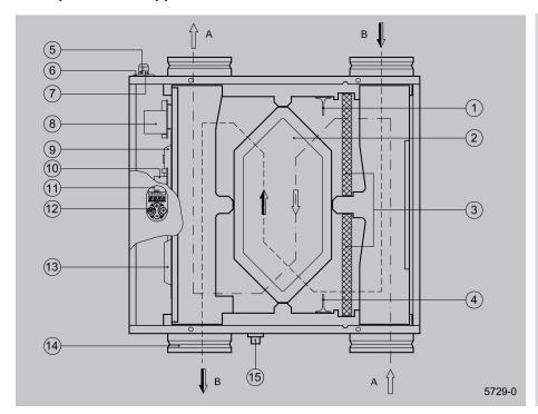
A= Output air flow B= Input air flow
