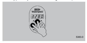
22 After cleaning the filter or a placing a new filter, the filter indication must be reset by pressing key "OK" during second
