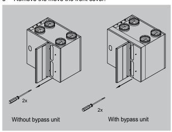
4 If the appliance is equipped with the optional bypass unit, it must now be removed.
