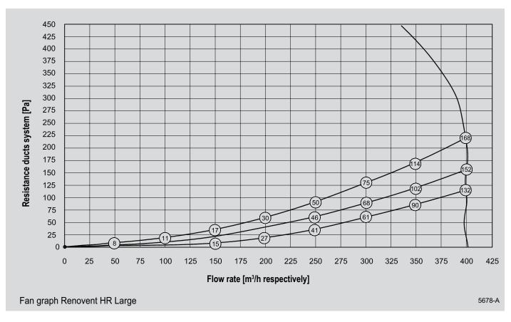
Note: The value stated in the circle is the capacity per fan (in Watt)
