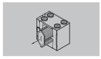
6 Clean the heat exchanger using hot water (55°C max.) and a regular detergent. Rinse the exchanger with hot water. If the appliance came ex factory with a bypass, then first remove the valve control device from the sliding grate.
