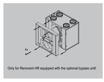
Remove the heat exchanger. Be careful not to damage the foam parts in the appliance.
